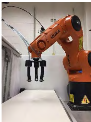
Figure 11. KUKA and conveyor – the core of kitchen assistant.
