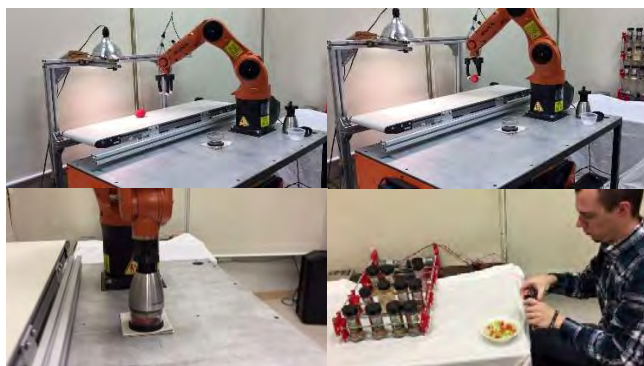
Figure 12. Salad preparation using the kitchen assistant. Top left: tomato entering system on conveyer. Top right: robot arm grasps tomato with three-fingered adaptive gripper. Bottom left: robot chops tomato with chopping tool. Bottom right: human uses spice rack element to season salad.
