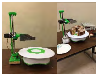
Figure 9. Robot structure with slicer, turntable, and cake.
